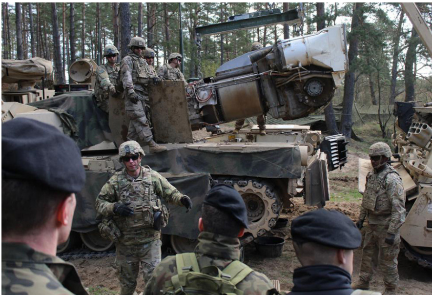
Figure 2. SSG Daniel S. Allen, a Bravo Company motor sergeant assigned to 1 st Infantry Division's 2 nd Battalion, 34 th Armored Regiment, teaches Polish soldiers the process of powerpack removal for an M1A2 Abrams tank as part of AOS at Bucierz Range, April 27, 2022. The 1 st Infantry Division is among other units assigned to V Corps, America's forward-deployed corps in Europe that works alongside NATO allies and regional security partners to provide combat-credible forces. (U.S. Army National Guard photo by SPC Hedil Hernández)
